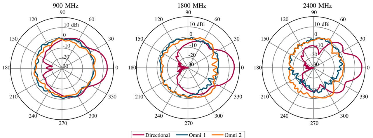
Fig. 3. Horizontal cut of the antenna gain patterns at an elevation angle  $\Theta = 15^\circ$  above horizon for 900 MHz (left), 1800 MHz (center) and 2400 MHz (right). Azimuth  $\Phi = 0^\circ$  is facing towards the front of the car.
