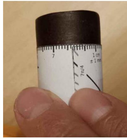
Fig. 3. Banknotes are augmented with rulers. a) 50 Euro prototype with a ruler along the top edge. b) A banknote measures the length of a protruding pipe. c) A prototype is used as measuring tape to determine the circumference of a metal rod.
