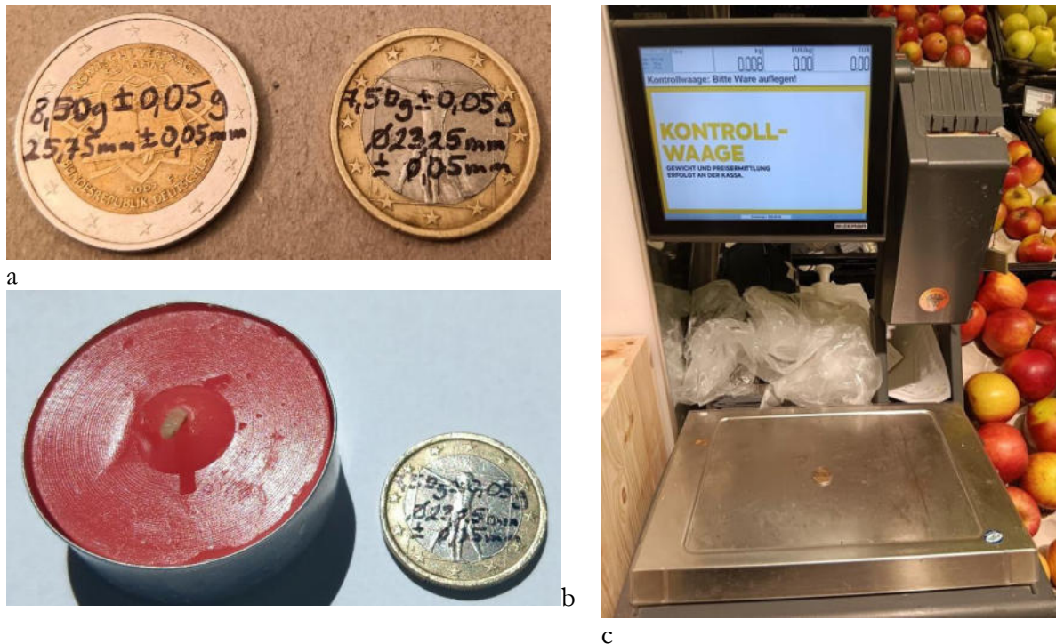
Fig. 7. Simple augmentations that can be added on any existing coins. a) Prototypes of 1 and 2 Euro coins that are labeled with mass and diameter. b) Use case: Coins for size comparison. The size comparison works as usual, and the inscription is useful for people who are not familiar with the currency. c) Use case: Testing of scales to prevent fraud. A coin is placed on a scale in the produce section of a supermarket to validate it. The consumer compares the value on the scale to the value on the coin.
