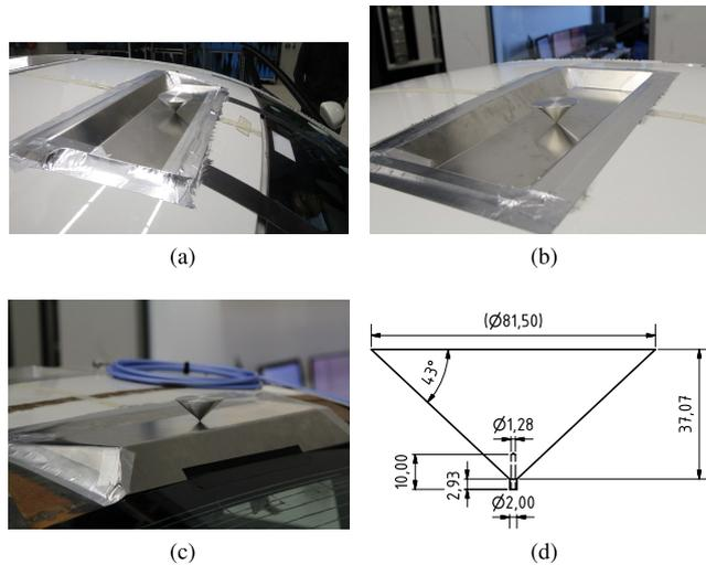
**FIGURE 2.** a) Antenna module on the front roof end above the windshield. b) Chassis antenna cavity in the roof center. c) Antenna shelf at the rear roof end. d) Cross section of the wideband conical monopole antenna. (Drawing reused with permission from [31], ©2018 IEEE.) All dimensions are in millimeters.
