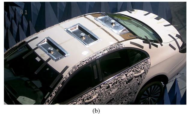
**FIGURE 1.** a) Sketch of the proposed antenna roof. b) Photograph of the antenna roof prototype on a sedan type passenger car mock-up. Antenna modules are located at the front, center and rear of the roof. All dimensions are in millimeter.
