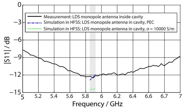
Fig. 4: Measured  $|S_{11}|$  compared to simulation results.
