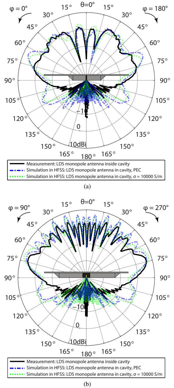
Fig. 6: Monopole antenna for 5.9 GHz inside a chassis antenna cavity. Simulation compared to measurement. Vertical cuts of the gain patterns along the a) short cavity side and b) long cavity side.
