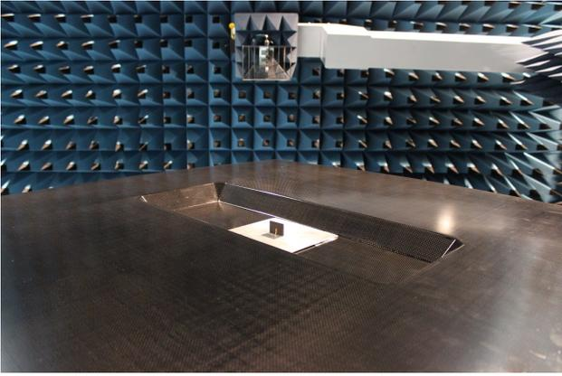
Fig. 2: Measurement of the monopole antenna for 5.9 GHz inside a CFRP chassis antenna cavity.
