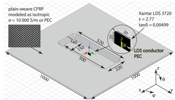
Fig. 1: Simulation model of a chassis cavity with a laser direct structured (LDS) monopole antenna for 5.9 GHz. All dimensions are in millimeter.
