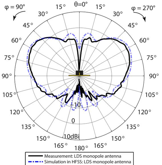
Fig. 3: Gain pattern of the LDS monopole antenna for 5.9 GHz without the cavity on a small  $150 \times 150$  mm<sup>2</sup> ground plane.
