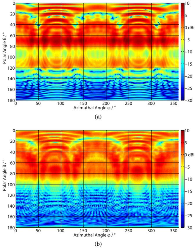
Fig. 5: Rectangular projections of the gain patterns. a) simulation with  $\sigma = 10000\text{S/m}$  and b) measurement
