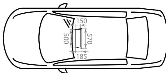
Fig. 1. Sketch of a chassis antenna cavity above the windshield on a sedan type vehicle. Dimensions are in millimeters.
