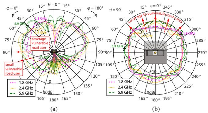
Fig. 7. Comparison of the measured gain patterns between the proposed cavity above the windshield and the cavity for the roof center (solid transparent lines, [11]); realized gain; linear polarization in  $\theta$  direction; a) vertical cuts front/back and b) horizontal cuts for polar angle  $\theta = 90^\circ$ .
