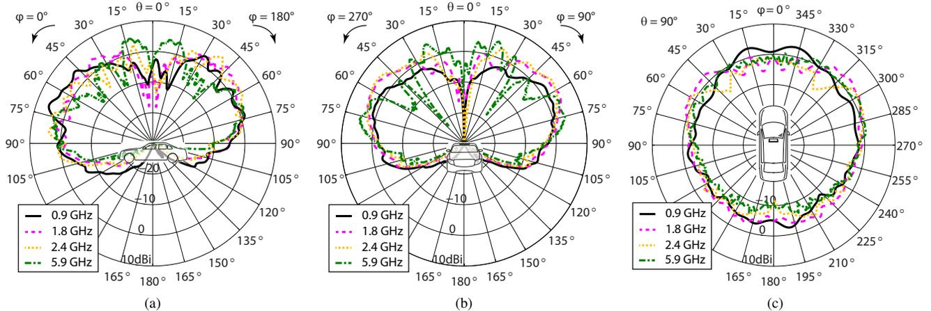
Fig. 6. Cuts of the measured gain patterns in situ on a sedan; realized gain; linear polarization in  $\theta$  direction; a) vertical cuts front/back b) vertical cuts left/right and c) horizontal cuts for polar angle  $\theta = 90^\circ$ .
