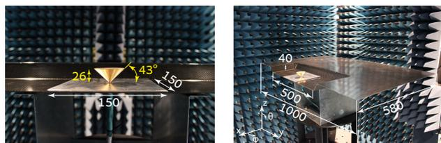
Fig. 2. Conical monopole antenna in the CFRP chassis antenna cavity that is open towards one side. Dimensions are in millimeters.
