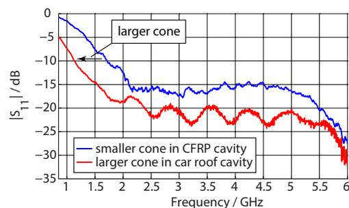
Fig. 4. Measured matching of the monocone antennas in the CFRP cavity and in the car roof. A larger cone was used for in situ measurements to obtain results for the lower LTE bands.
