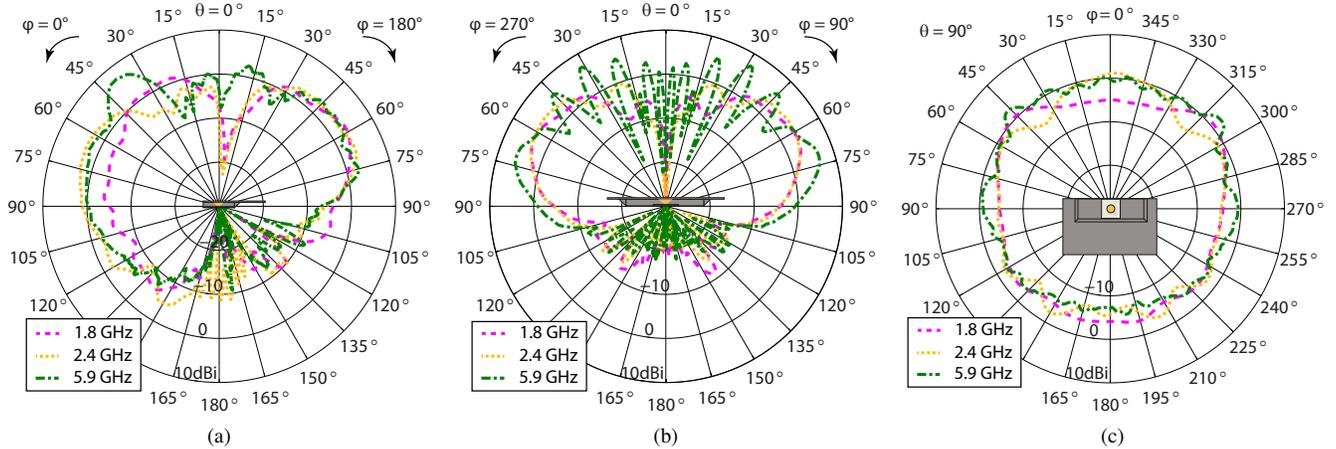
Fig. 5. Cuts of the measured gain patterns in the CFRP cavity; realized gain; linear polarization in  $\theta$  direction; a) vertical cuts front/back b) vertical cuts left/right and c) horizontal cuts for polar angle  $\theta = 90^\circ$ .
