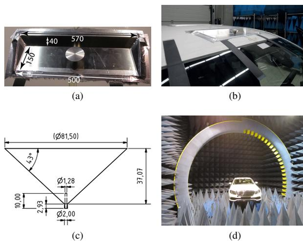
Fig. 3. a) Antenna cavity adapted to the roof curvature. b) Prototype of the antenna cavity located above the windshield. c) Dimensions of the larger cone for the car prototype. d) Measurement in VISTA. Dimensions are in millimeters.
