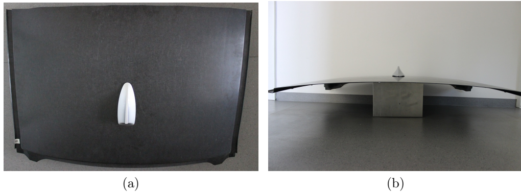
Figure 2.17: Shark-fin automotive antenna module on half of a CFRP car roof: a) top view and b) front view.
