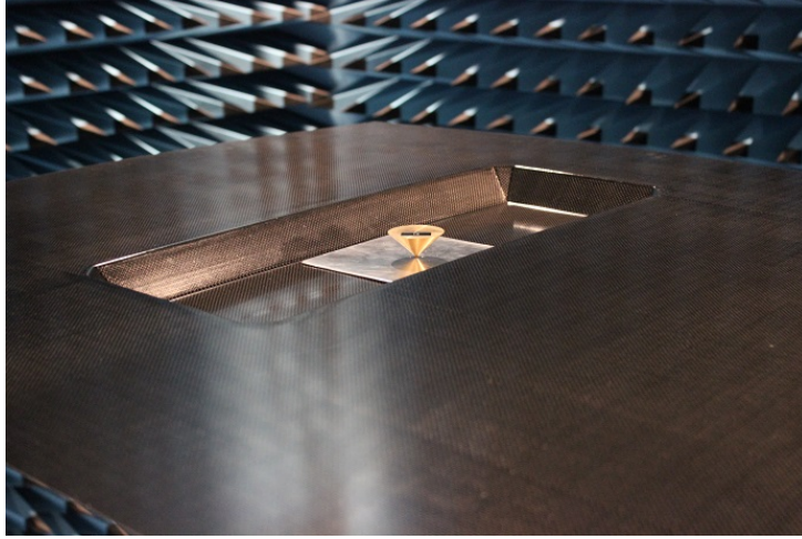
Figure 3.9: A conical monopole antenna inside the chassis antenna cavity.
