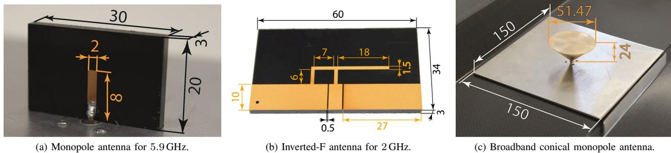
Fig. 2: Dimensions of the antenna prototypes measured inside the chassis antenna cavity. All dimensions in millimeter.
