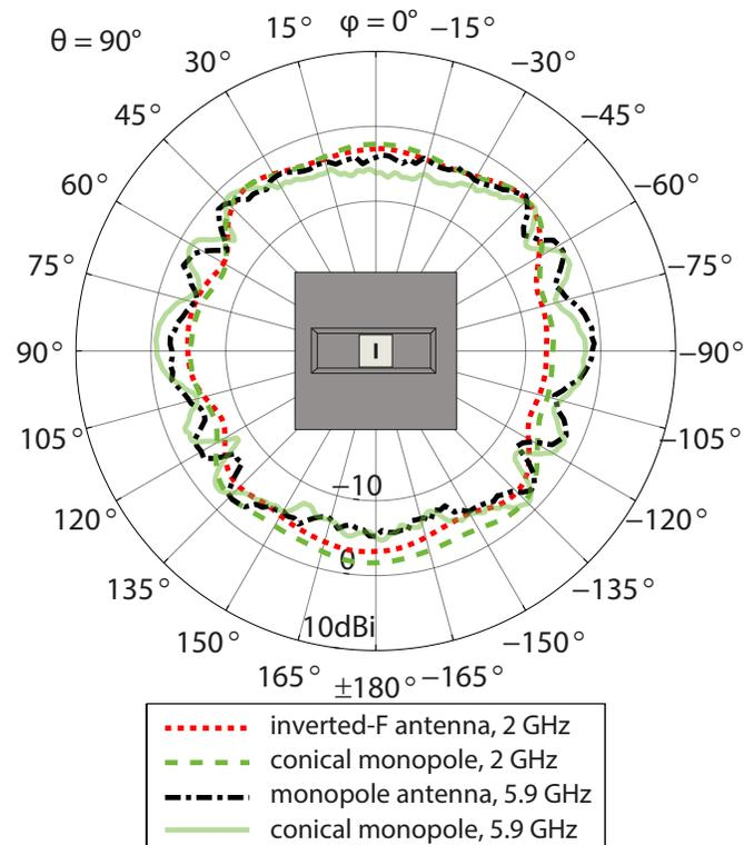
Fig. 7: Measured gain patterns of the IFA at 2 GHz and the monopole antenna at 5.9 GHz inside the cavity, horizontal cut for  $\theta = 90^\circ$ .
