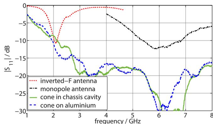
Fig. 4:  $|S_{11}|$  of the inverted-F antenna and the monopole antenna inside the cavity.
