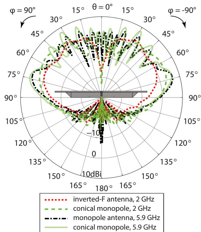
Fig. 6: Measured gain patterns of the IFA at 2 GHz and the monopole antenna at 5.9 GHz inside the cavity, vertical cut for  $\varphi = 90^\circ$ .
