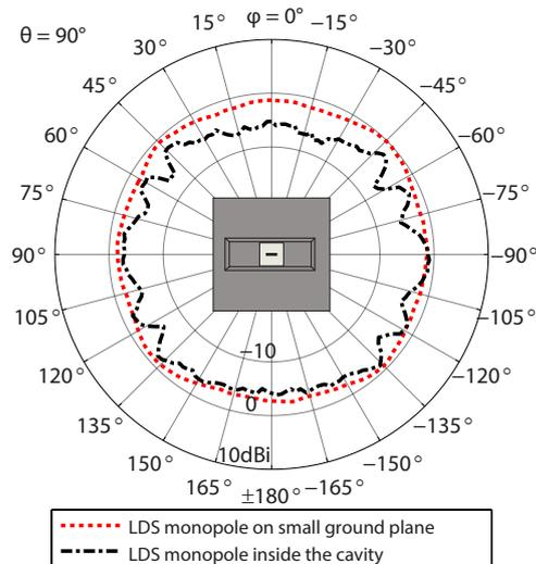
Figure 6: Horizontal cut of the gain pattern dependent on azimuthal angle  $\varphi$  for  $\theta = 90^\circ$
