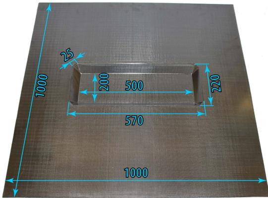
Figure 1: CFRP prototype of the antenna module, debugged specimen after the curing in the autoclave. All dimensions are in millimeter.
