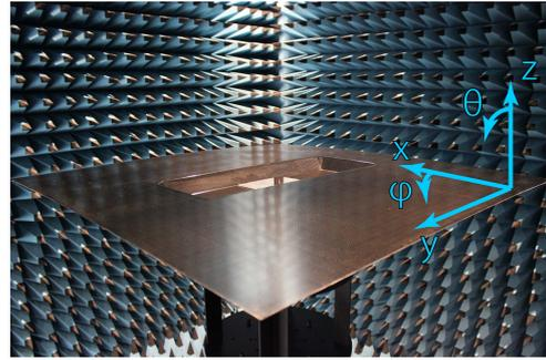
Figure 2: LDS monopole antenna inside the CFRP integrated chassis module. The depicted coordinate system is displaced to increase visibility, the origin is in the center of the cavity.
